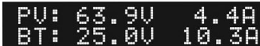
Figure 4-3 PV panel and battery charge status display interface
